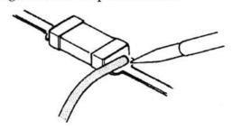
Grasp the chip on both sides with tweezers, and gently twist the tweezers back and forth (to break the adhesive bond) while alternately heating each electrode. Be careful to avoid peeling the foil traces from the board.
